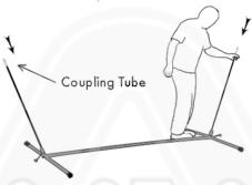
Install two lower Black Rods with Coupling Tubes up, in angled Pipes
