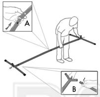
Join two straight Pipes together. Fig. A Then attach both end Legs. Fig. B
