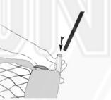
5. Take Black Rod and slot into lower 6. Hold Black Rod pulling Orange sleeve up and loop White Cord over rod top See #8.
