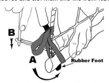
Finally take black Loops (A) and place under Rubber Feet. (B) Stake the Net on Grass or use Bowbags on Turf (not supplied)
